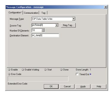
Complete the dialog box for the data area to be transferred. CIP Data Table messages require a tag database element for both the source and destination. The **SOURCE TAG** is a tag defined in the Controller Tag database. The **DESTINATION ELEMENT** is the tag element in the gateway.
