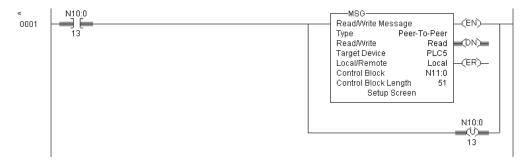
Set the **READ/WRITE** parameter to **READ.** The gateway supports a **TARGET DEVICE** parameter value of **500CPU** or **PLC5.** In order to complete the configuration of the MSG instruction, select the **SETUP SCREEN** area of the MSG object. This displays the following dialog box.
