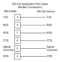
For most modem applications, RTS/CTS handshaking should be enabled in the port configuration.
