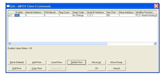
In order to interface the PLX30gateway with Modbus TCP/IP server devices, a command list must be constructed. The commands in the list specify the server device to be addressed, the function to be performed (read or write), the data area in the device to interface with and the registers in the internal database to be associated with the device data. The Client command list supports up to 16 commands per Client.
