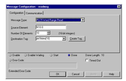
Complete the dialog box for the data area to be transferred. For PLC5 and SLC messages, the **SOURCE ELEMENT** should be an element in a data file (such as, N10:0). For the PLC2 Unprotected Read message, the **SOURCE ELEMENT** is the address in the gateway's internal database and cannot be set to value less than ten. This is not a limitation of the gateway but of the RSLogix software. The **COMMUNICATION** information must also be configured. An example of the dialog box follows:
