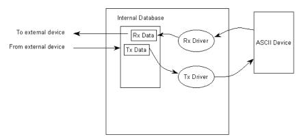
Data received from the ASCII device is accepted by the receive driver and placed in the receive database location configured by the user. The receive driver waits until the user-configured termination condition is recognized while receiving the data before placing the new data into the database.
