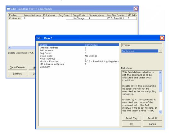
**5** When configuration is complete, download the configuration to the gateway.
