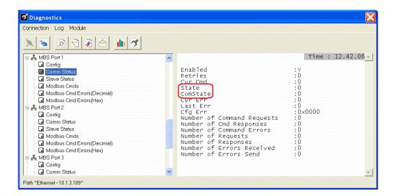
These status values are state registers. They are used as 'scratchpad' areas by the operating firmware to keep track of the current logical state of activities on a slave port. These state registers are constantly changing as the gateway progresses through the various stages needed to process communication on the serial ports. This processing happens faster than can be followed, unless a port error causes the value to remain constant for some noticeable length of time.
