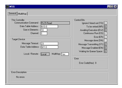
The **TARGET DEVICE DATA TABLE ADDRESS** must be set to a valid file element (such as, N11:0) for SLC and PLC5 messages. The **MULTIHOP** option must be set to **YES**.
