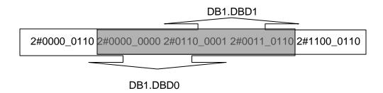
The gray area above represents the byte memory locations being overlapped when double word address is used consecutively (DB1.DBD0, DB1.DBD1, DB1.DBD2, etc).
