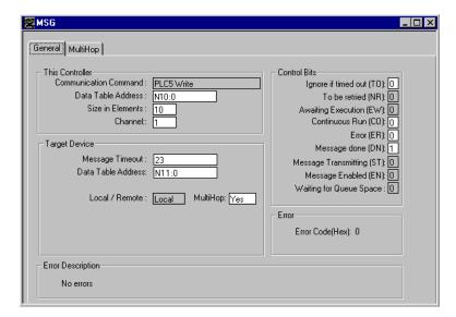
The **TARGET DEVICE DATA TABLE ADDRESS** must be set to a valid file element (such as, N11:0) for SLC and PLC5 messages. The **MULTIHOP** option must be set to **YES**. The **MULTIHOP** tab portion of the dialog box must be completed as displayed in the following window:
