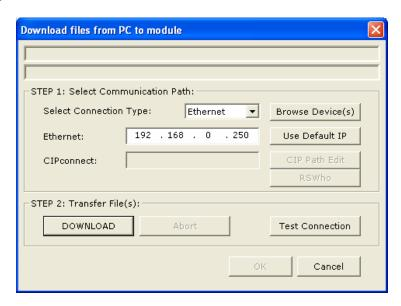
3 Click the **BROWSE DEVICE(S)** button to launch the *ProSoft Discovery Service* window, which displays the ProSoft devices on the network and their IP addresses.
