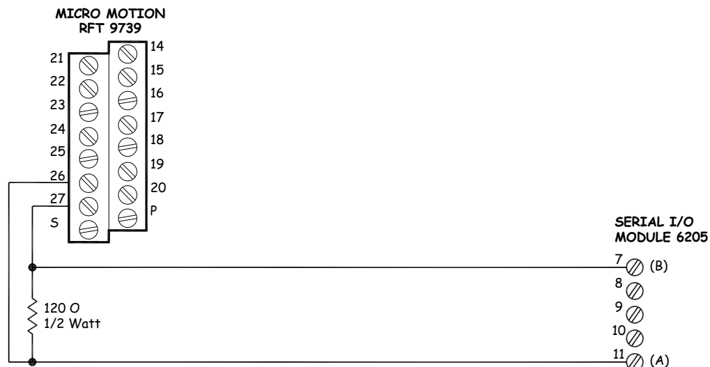
Figure 68. Wiring a RFT9739 via two wire RS 485 Communications
