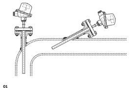
The situation described in the classical temperature measurement setup shows that contact with the measuring medium can bring a wide array of difficulties. These difficulties have to be mastered for reliable and, above all, safe system operation, which leads to high costs [1].
