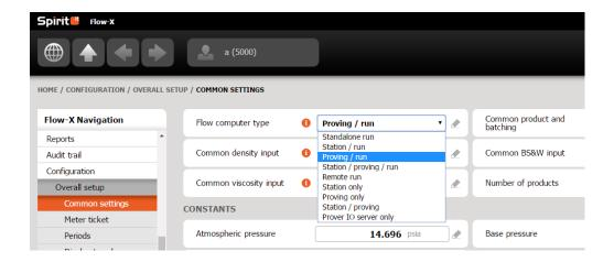
When upgrading a flow computer from a previous application version to this new version, please remember to set this parameter accordingly.
