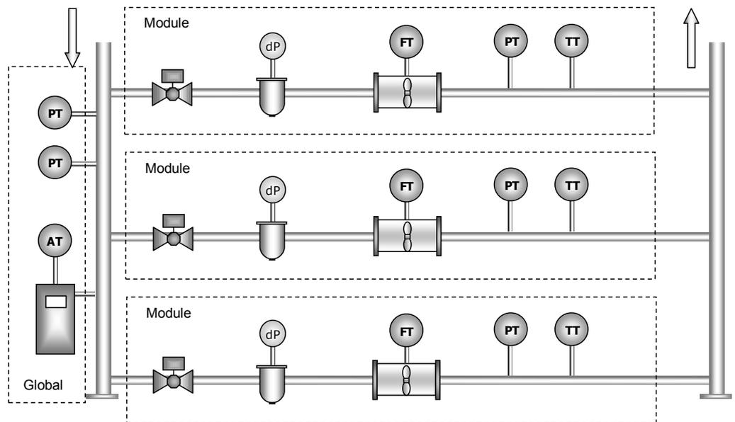
Figure 3: Typical gas metering station
