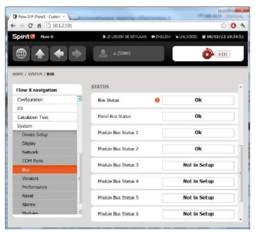
Figure 12: Checking the communication bus status
