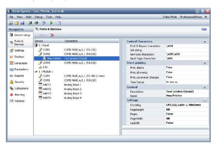
Figure 17: Serial printer settings
