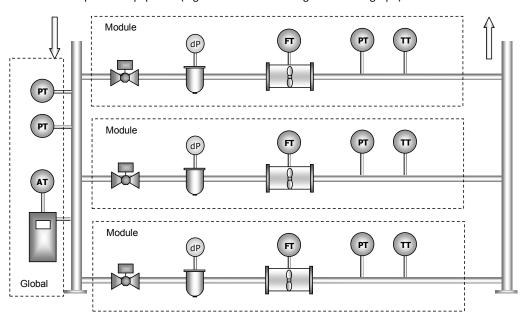
Figure 3: Typical gas metering station
