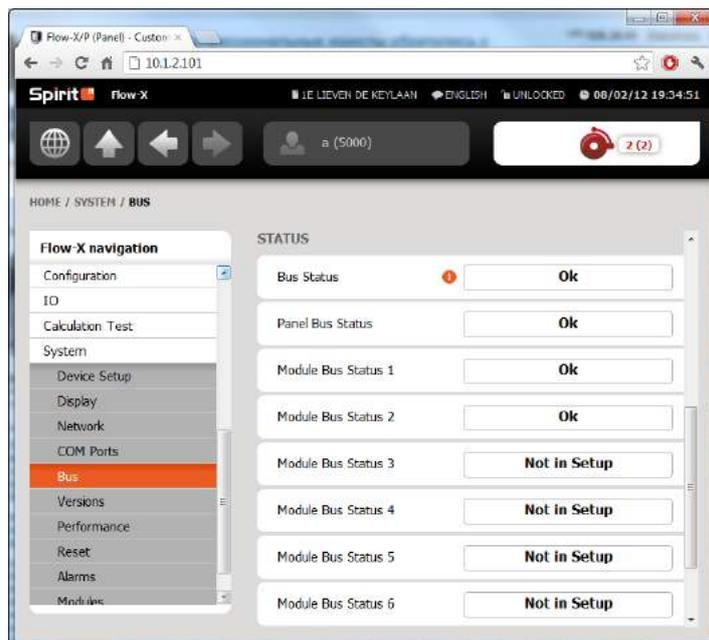
Figure 12: Checking the communication bus status
