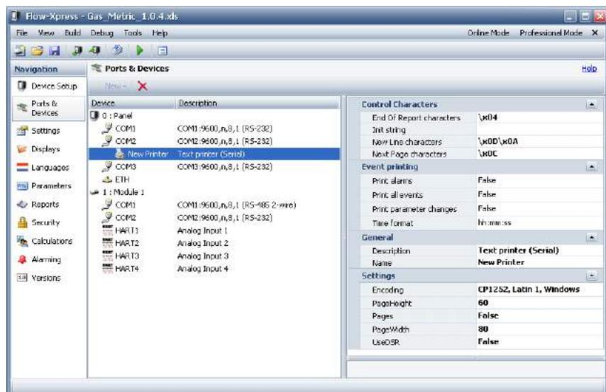
Figure 17: Serial printer settings
