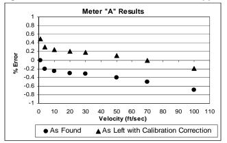
Figure 1. Meter "A" Results with Correction Applied.
