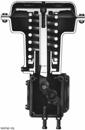
Figure 3-34. Diaphragm Actuator for Rotary Shaft Valves
