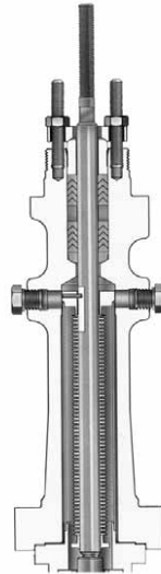
Figure 1-6. Bellows Seal Bonnet
