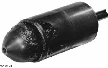
Figure 5-6. Typical Appearance of Flashing Damage
