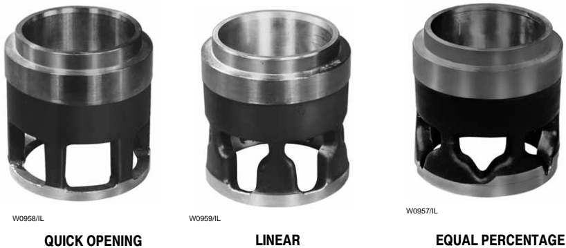
Figure 1-8. Characterized Cages for Globe-Style Valve Bodies
