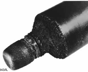
Figure 5-7. Typical Appearance of Cavitation Damage
