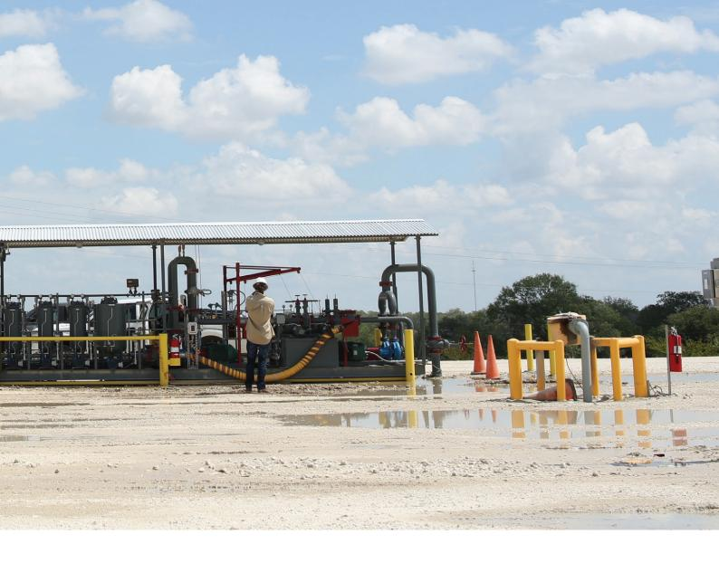
eXSite is specifically made to automate and regulate the movement of crude oil from the production area to gathering facilities and oil terminals. Field run and LACT tickets are almost instantly available to the back office and automatically emailed to customers.
