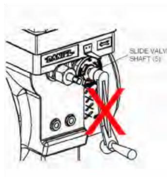
Figure 4-1 Top (14) KEEP OUT ZONE* Figure 4-2 Improper Location of Operating Wrench (2) During an Orifice Plate Change Operation
