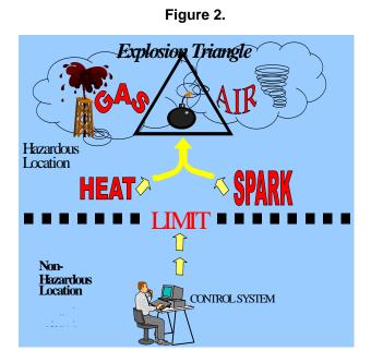
If the hazardous location is defined as the explosive triangle, then the I.S. barrier device limits the electrical energy that may transfer as either heat or spark to the combustible location.
