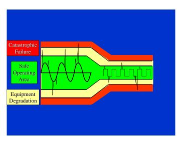
The result of repeated "attack" on solid state devices present in nearly all hydrocarbon measuring instruments by transients at the degradation level are unexplained "clear blue day" failures and significantly reduced Mean Time Between Failure (MBTF) of the equipment.
