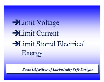
How is this limitation accomplished and how can it practically be applied to the typical 4-20mA current loop?
