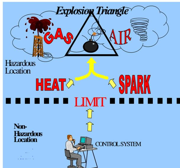
If the hazardous location is defined as the explosive triangle, then the I.S. barrier device limits the electrical energy that may transfer as either heat or spark to the combustible location.
