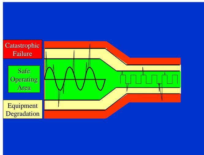
The result of repeated “attack” on solid state devices present in nearly all hydrocarbon measuring instruments by transients at the degradation level are unexplained “clear blue day” failures and significantly reduced Mean Time Between Failure (MTBF) of the equipment.
