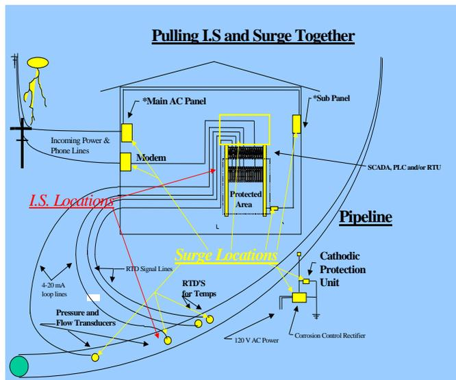
Closer inspection of Figure 11 reveals that some of the very same areas and instruments vulnerable to lightning and surge damage are the same areas requiring intrinsically safe barrier protection.
