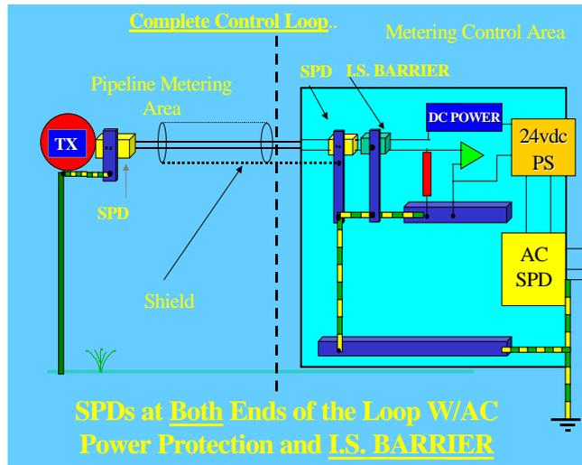
Now all the elements of the control system beginning with the field transmitter, the wiring, the intrinsically safe barriers, the PLC I/O, in addition to the DC and AC power supplies are continuously shielded from explosion or the ravages of lightning and surge.
