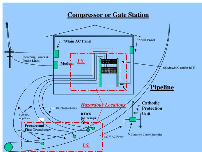
These field-mounted instruments must communicate with the PLC, SCADA, or RTU control systems located remotely in the station via wiring, normally 18AWG TSP
