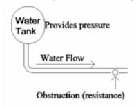
This relationship could be expressed mathematically as the flow (current) is equal to the pressure (Volts) divided by the resistance to flow (ohms). This is Ohm's law.
