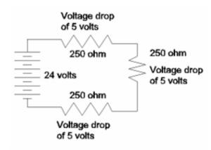
This is a quick rule of thumb. The actual loads would include the power (i.e. voltage drop) of the transmitter and the resistance of the wire. This assumes a two-wire transmitter. The resistance of the wire can be calculated from the manufacture data sheet, a table from a National Electrical code book, or just read with an ohmmeter. If calculated from a data sheet or table, remember to multiply this resistance by two. This is because of the two legs (out to and back from the transmitter).
