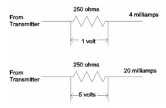
The question would be raised here of what does that have to do with the supply voltage. Remember Kirchhoff's voltage law. It states that the sum of the voltage drops around a series circuit must equal the supply voltage. This becomes very important in this application. This sample application will use 12 Volts as the supply and three loads of 250 ohms each.
