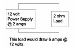
This would create an over current condition that would cause the power supply fold over. Probably the supply voltage would drop to less than a Volt.
