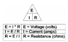
Voltage equals the current times the resistance. Current equals the voltage divided by the resistance and resistance equals to the voltage divided by the current. One of the important things to remember is the relationship between current and resistance. It is an **inverse** relationship. What this means is as resistance goes up the current goes down.
