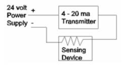
The supply voltage will determine the number of loads. A brief explanation is in order here. The most common load is 250 ohms. The reason is most receivers actually read the information as 1 to 5 Volts. This works by a method that can be explained by ohms law. The formula we are interested in here is E (Volts) = I (current) \* R (resistance). The current 4 milliamps (.004 Amps) \* 250 ohms equals 1 Volt. The top end of 20 milliamps (.020 Amps) \* 250 ohms equals 5 Volts.
