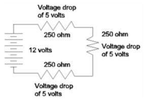
The loads drop 5 Volts each. Three loads times 250 ohms would equal 15 Volts. This exceeds the supply voltage. Clearly this application would not work. The application using 24 Volts as the supply voltage would work since 24 Volts - 15 Volts equals 9 Volts left.
