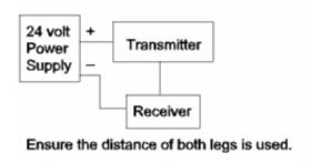
Always remember to read the data sheets for the receiver. The most common load is 250 ohms however this isn't the only load size. There are receivers that have fractional loads. It is possible that the receiver could require the input to be scaled to something other that 1 to 5 Volts.
