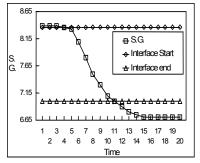
The "cut" can be made manually or automatically. If the "cut" is made automatically then it important that any S.G within the interface which lies within a product SG band is not flagged as new product. To ensure this does not happen it is normal to measure SG and rate of change of SG. The change from product to product is as follows:
