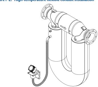
Figure F-2: High-temperature flexible conduit installation
