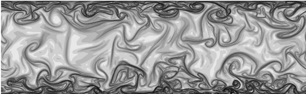
**Figure 2 - Turbulence within the Flowstream for Reynolds Number Greater than 10-12,000**
