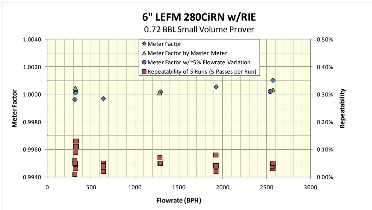
**Figure 8 – Linearity and Repeatability Results of 6" Reducing Nozzle Meter with the RIE (Caldon LEFM 280CiRN)**
