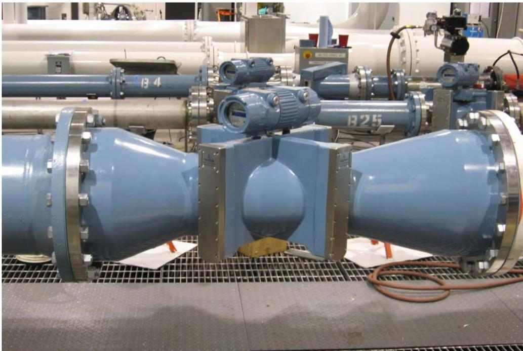
**Figure 9 - 16" Reducing Nozzle Meter (Caldon LEFM 280CiRN)**
