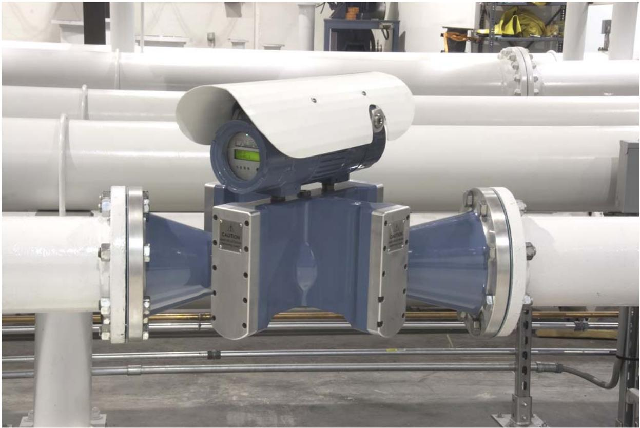
Figure 5 - Reducing Nozzle Meter (Caldon LEFM 280CiRN)
