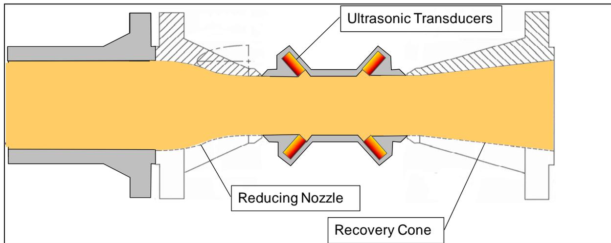
**Figure 4 - Reducing Nozzle 8-path Meter**
