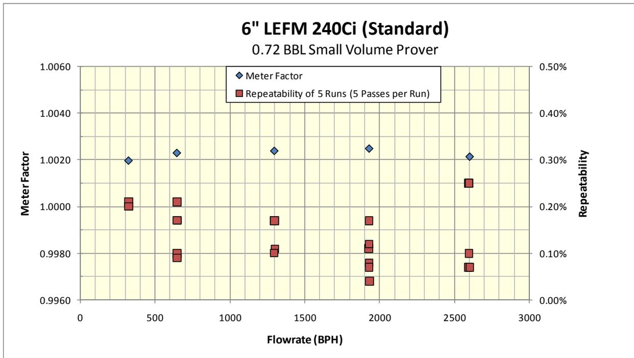
**Figure 3 – Linearity and Repeatability Test of 6" Four-path Ultrasonic Flowmeter (Caldon LEFM 240Ci)**
