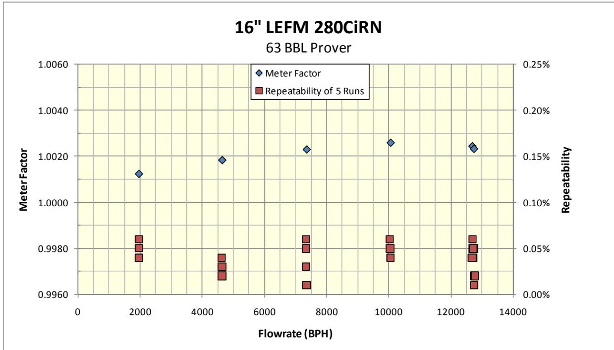
Figure 10 – Linearity and Repeatability Results of 16" Reducing Nozzle Meter (Caldon LEFM 280CiRN)
