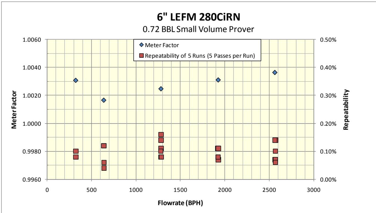
Figure 6 - Linearity and Repeatability Results of 6" Reducing Nozzle Meter (LEFM 280CiRN)
