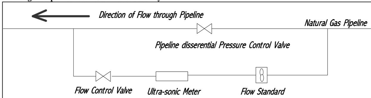
**Drawing 2. Pressurized Loop Based Calibration Facility.**
