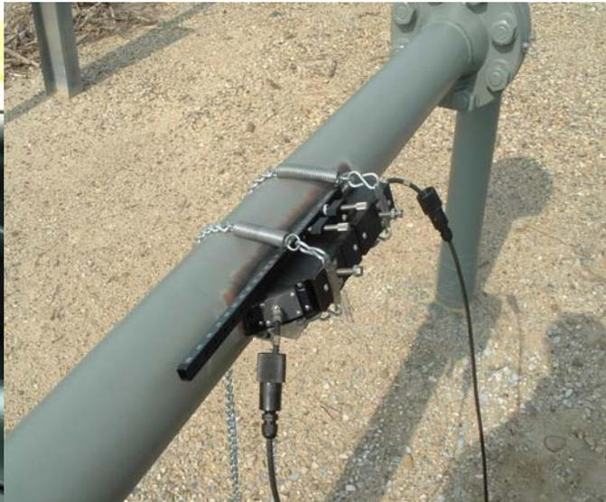
The applications for the use of these meters in the petroleum arena has continued to grow and includes highly aerated liquids, high viscosity liquids ( 4000 cp ), hydraulic lines and additives in addition to crude oils and refined products. Because of their portability and easy of installation they are easily used in line displacements and re-filling. There is a lot of truth to the say if you can flow it in a pipe, it can be measured with an ultrasonic meter.
